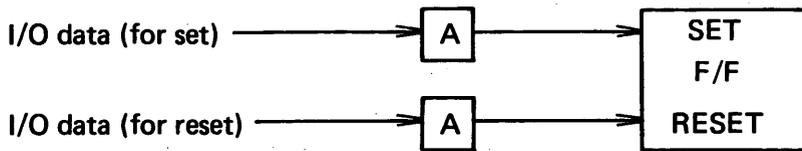
When I/O data for set are input, internal flip-flop is set. When I/O data for reset are input, flip-flop is reset.
