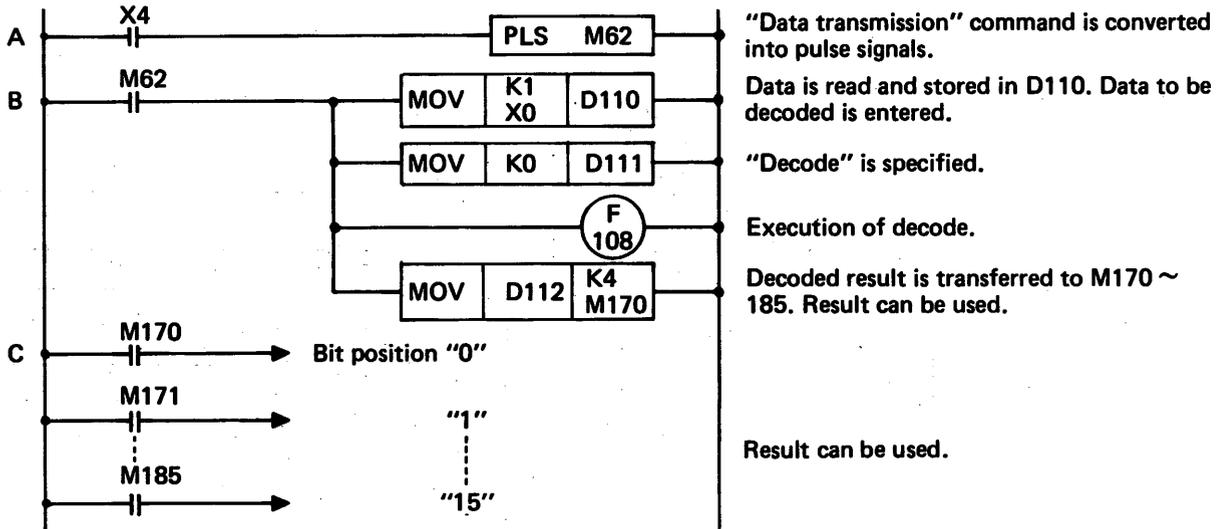
Fig. 5.4.12.3 Decode Circuit Composition
