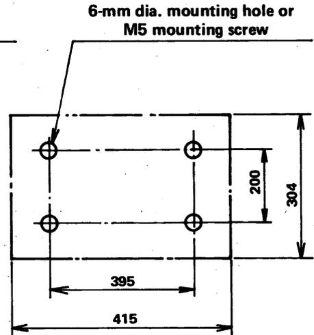
Fig. 8.2.7 Mounting Dimensions of K68B
