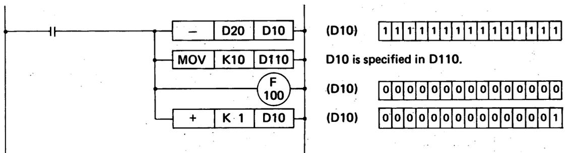
Fig. 5.4.14.2 Data Inversion Circuit
