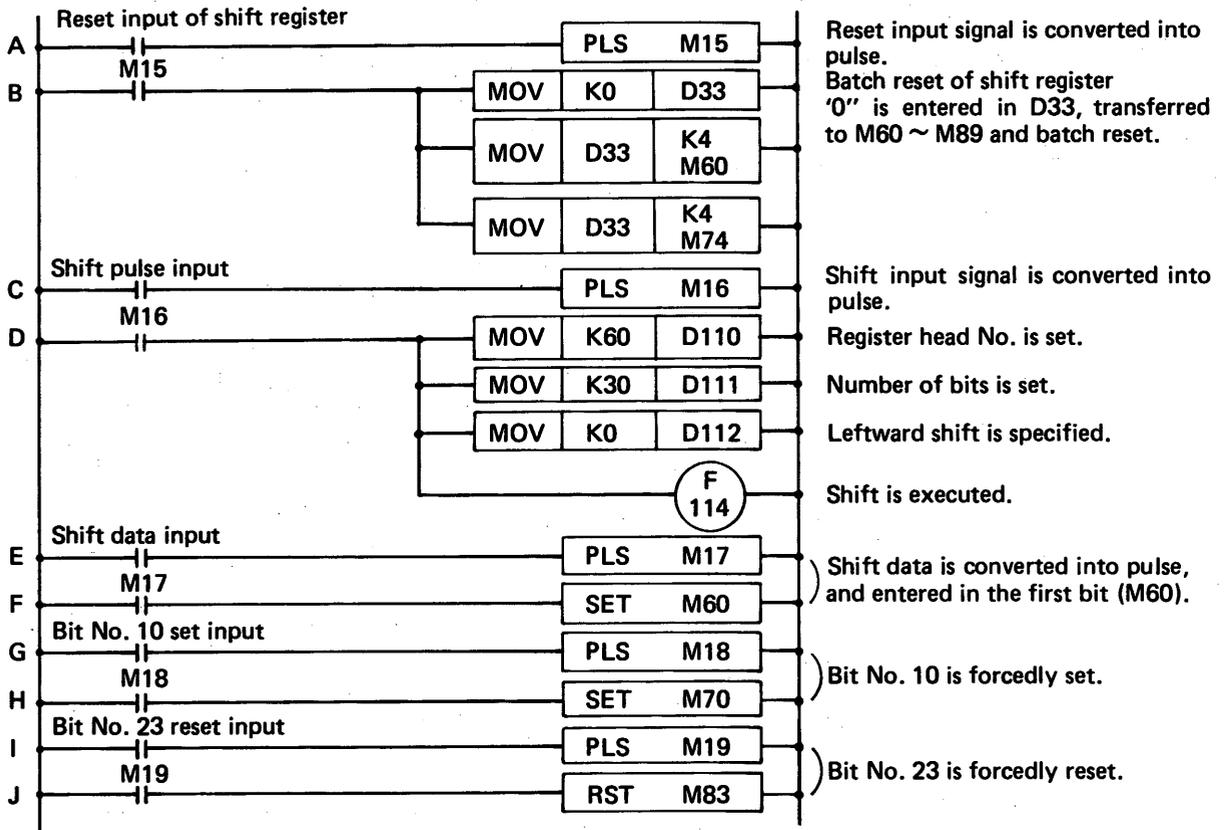
Fig. 5.4.6.4 Leftward Shift Register Circuit
