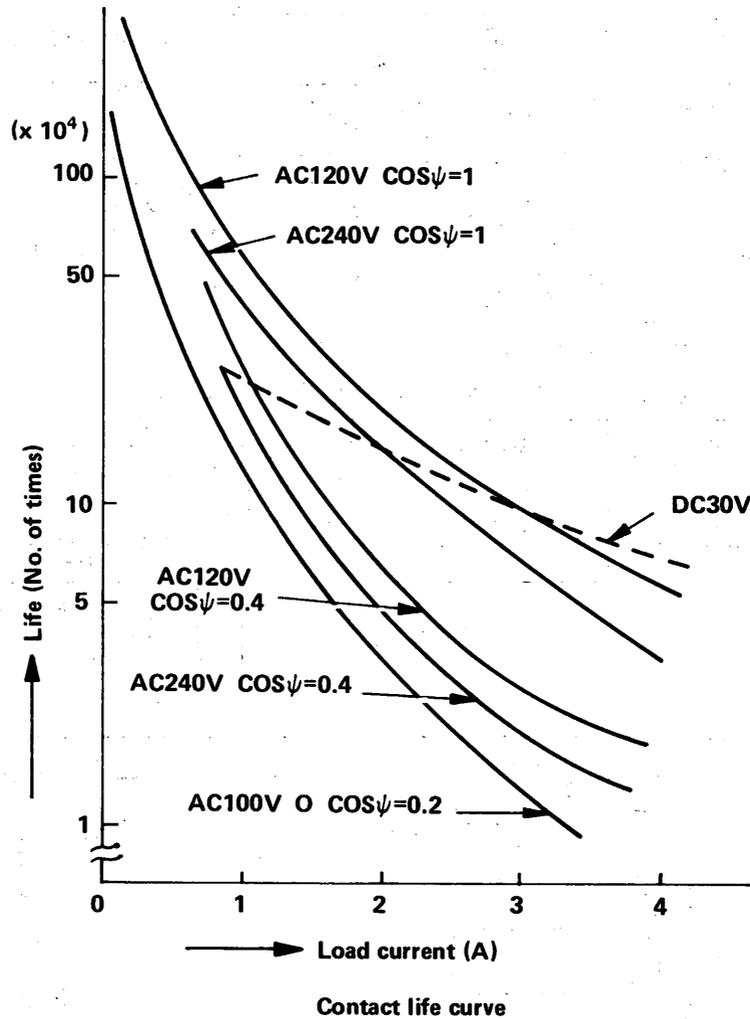
*Note: When DC 100V load is opened and closed at the contact, set load current at 0.1 A or lower. When frequency is too high even at 0.1 A load, be sure to connect C-R surge killer or flywheel diode in parallel with the load.*
