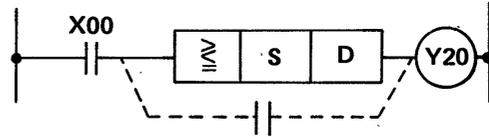
The compare instruction is equivalent to contact in handling. However, since OR instruction cannot be performed, do as shown below.
