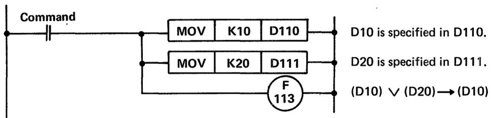
Fig. 5.4.5.2 16-bit data OR operation circuit
