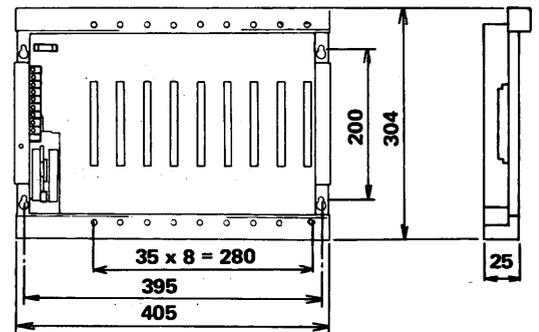
Fig. 8.2.4 External Dimensions of K68B Extension Unit
