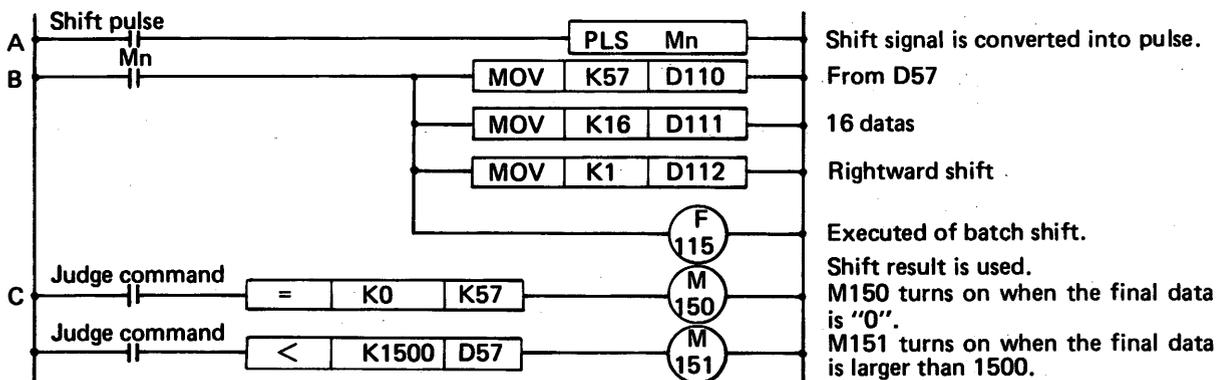
Fig. 5.4.7.3 Batch Shift Circuit Composition
