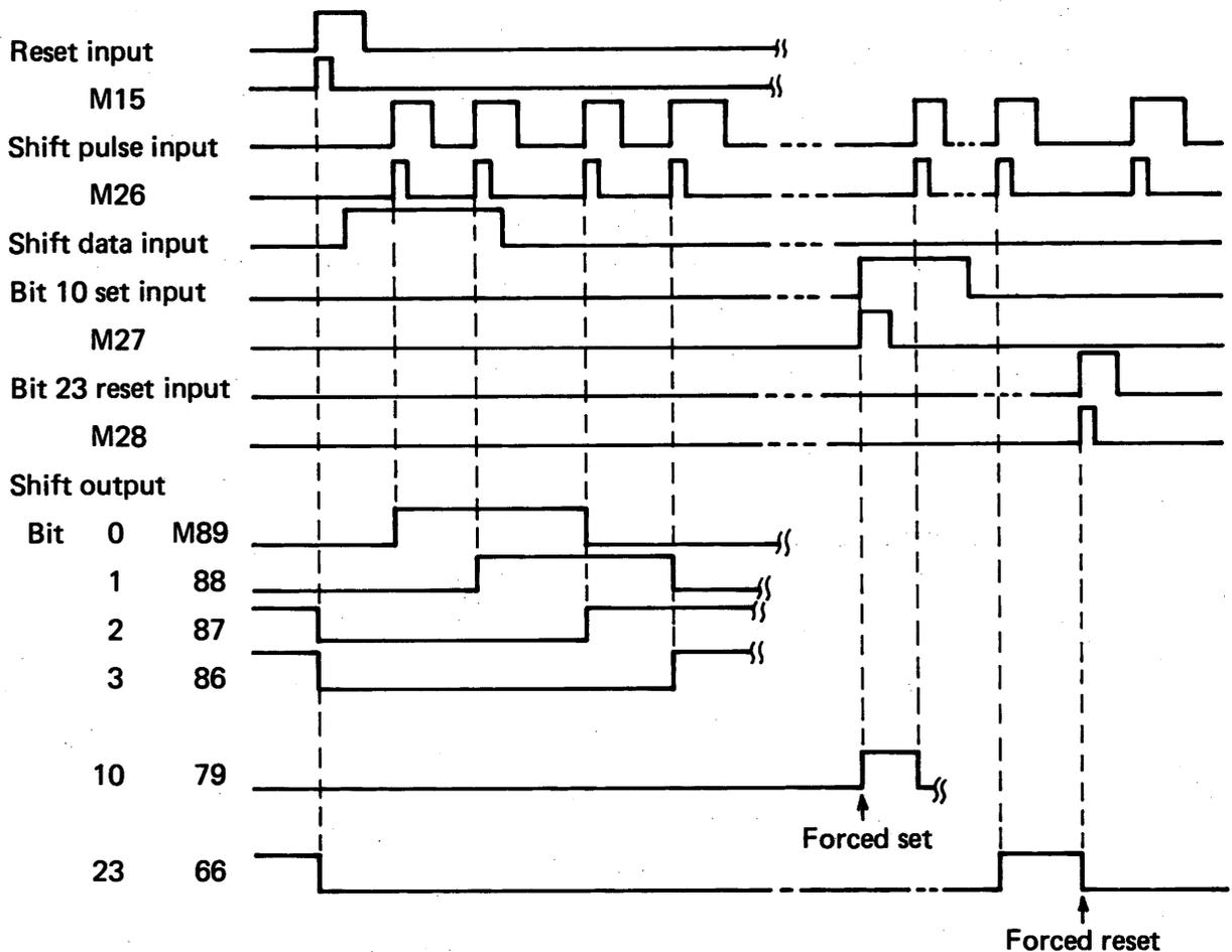
Fig. 5.4.6.8 Rightward Shift Register Timing Chart
