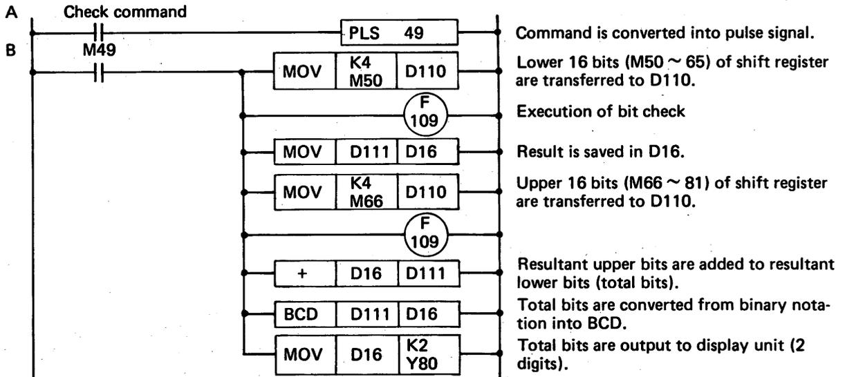
Fig. 5.4.13.2 Display of Number of Bits "1" in Shift Register
