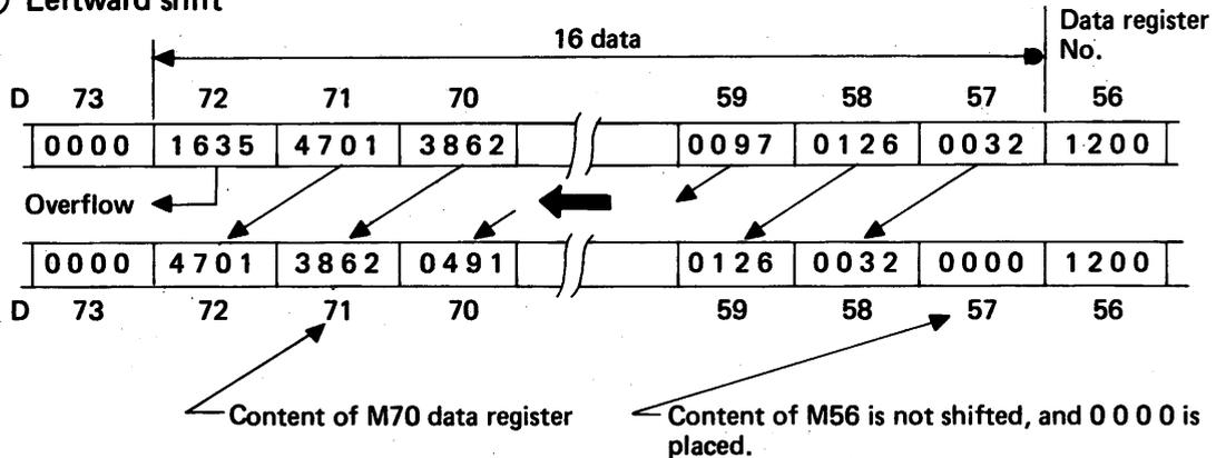
Fig. 5.4.7.1 Batch Shift (Leftward shift)
