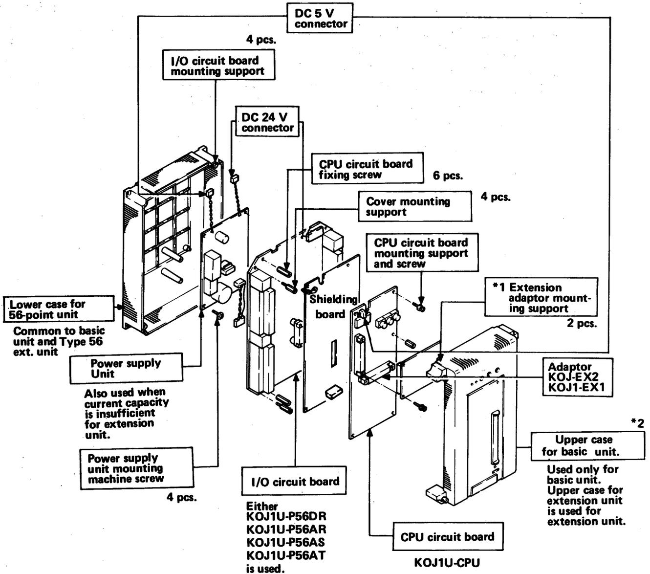
\*1 When extension adaptor is used, this support is utilized. Fit it with attached screws.
