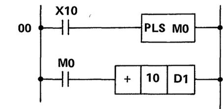
When M0 turns on, D1 is added to 10 and the value is entered into D1.
