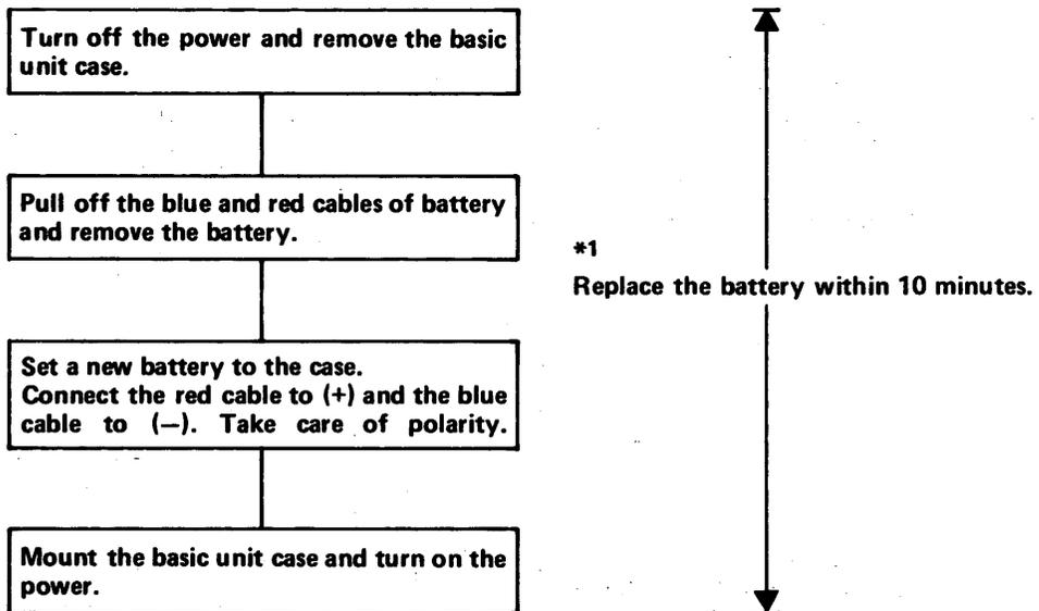
\*1 When the battery is changed, the time from when the power is turned off and the battery is changed to when the power is turned on again should be within 10 minutes. If it exceeds 10 minutes, enough care should be taken because the contents of program and latch function will be cleared.
