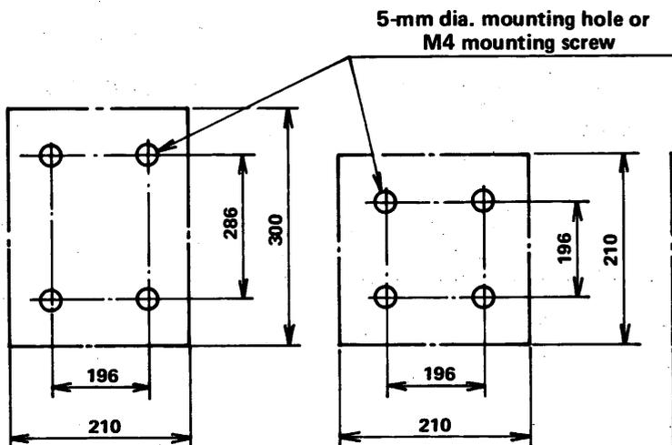
Fig. 8.2.5 Mounting Dimensions of Basic Unit and E56
