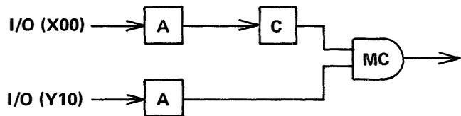
MC and MCR require index No. "Kn". Be sure to provide MCR Kn for MC Kn.
