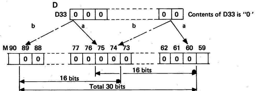
Fig. 5.4.6.5 Batch Reset of M
