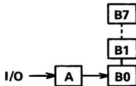
**LDI** Specific relay No. content is inverted and stored into register A.
