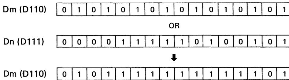
Fig. 5.4.5.1 16-bit data OR operation
