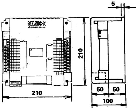
Fig. 8.2.3 External Dimensions of E32 Extension Unit
