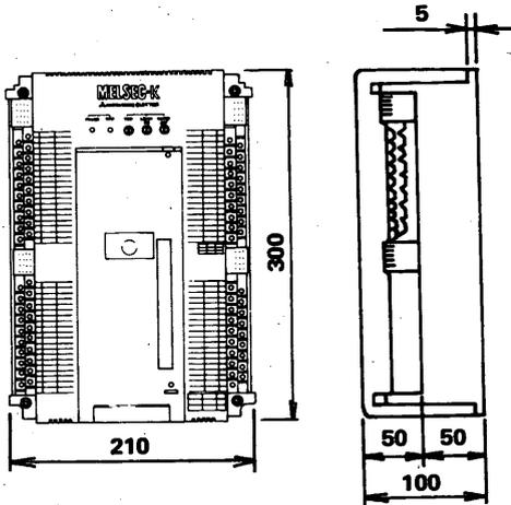
Fig. 8.2.1 External Dimensions of Basic Unit
