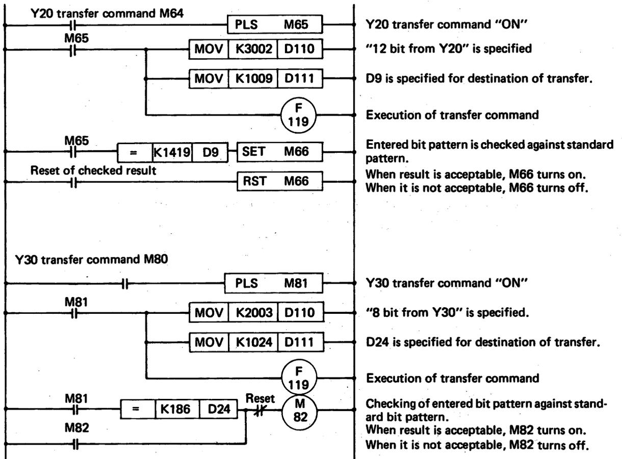
Fig. 5.4.11.2 Y → D Data Transfer Circuit.
