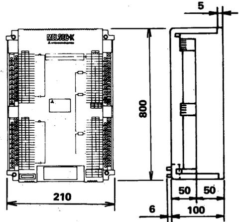
Fig. 8.2.2 External dimensions of E56 Extension Unit
