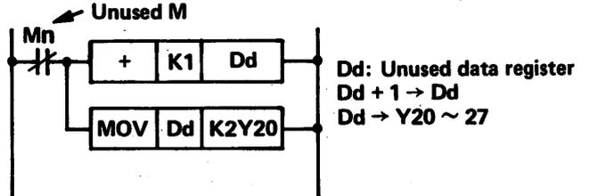
2. When the sequencer is run, Y20 to Y27 displays are indicated with 0 ~ 255 ~ 0. Therefore, measure the time T, i.e. from when Y20 to Y27 are all turned off to when they are all turned on again.
