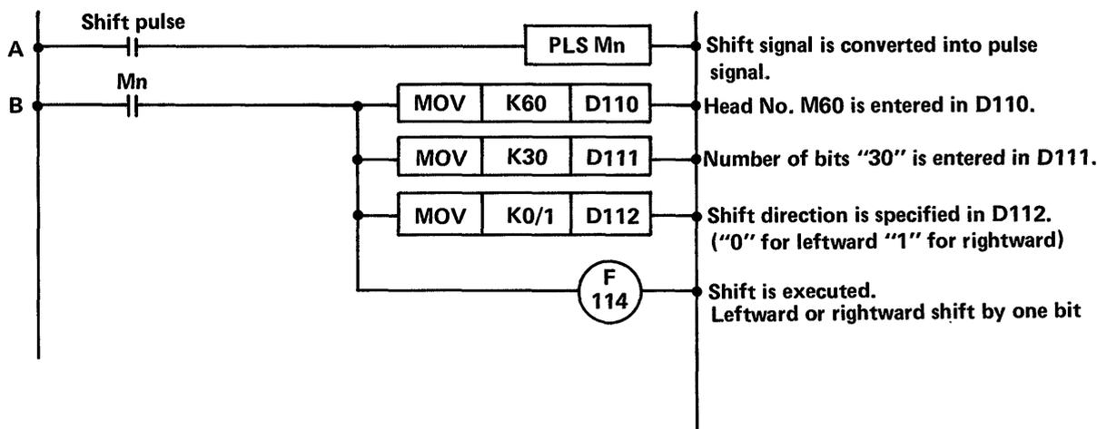
Fig. 5.4.6.1 Shift Register Circuit Composition
