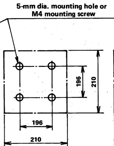
Fig. 8.2.6 Mounting Dimensions of E32
