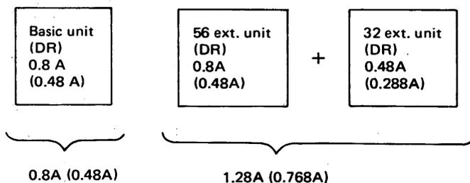
When capacity is calculated on the assumption that each unit has simultaneous 60% "ON" ratio, values in parentheses are obtained. In this case, power supply unit is added to the E56 extension unit in order to supply power also to the E32 extension unit.
