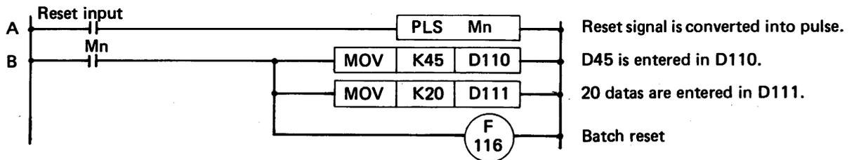
Fig. 5.4.8.2 Data Register Batch Reset Circuit
