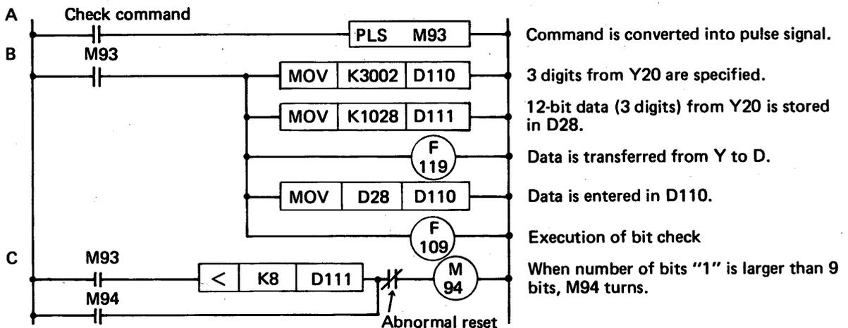
Fig. 5.4.13.3 Checking of Number of Bits "1" of Output Y
