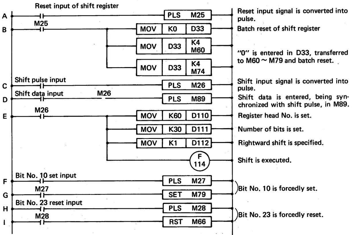
Fig. 5.4.6.7 Rightward Shift Register Circuit
